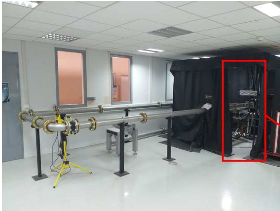
Current laser based velocimetry test configuration on MONT-BLANC
