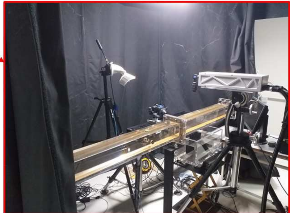
Square section Plexiglas pipe for future 3D3C PIV investigations (work in progress)
